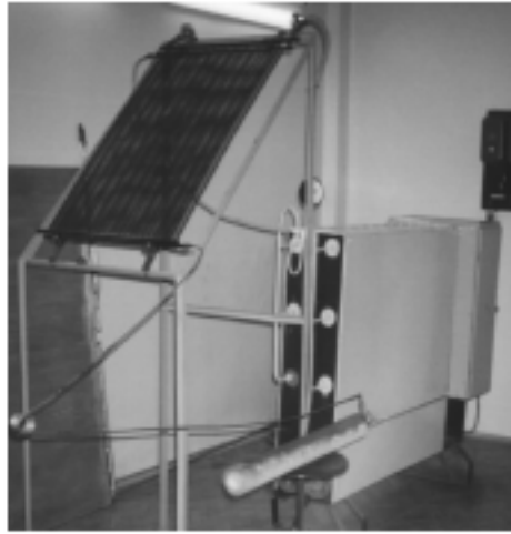
Fig. 8. General view of the sorption heat pump.
